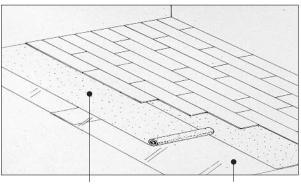
Pergo SilentStep<sup>™</sup> Foam or Soundbloc<sup>™</sup> Foam to be used with flooring that doesn't have attached underlayment. Vapor barrier over concrete – Moisturbloc™
