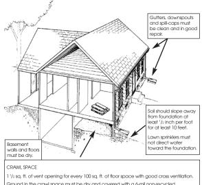
17/3 st, iii. Oi veni opening toi eveny too st, iii. oi noo space wiin good closs venination. Ground in the crawl space must be dry and covered with a 6-million-necycled (100% virgin) resin polyethylene film; seams overlapped at least 8 inches.
